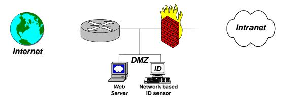
Figure 1 - Deploying 1 ID system
