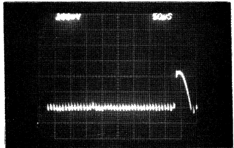
Output Voltage: 100mV/division 50 \mu s/division Step Load Change: 20A to 10A (b)
