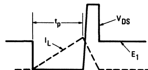
Fig. 2 – Clamped Inductive Waveforms
