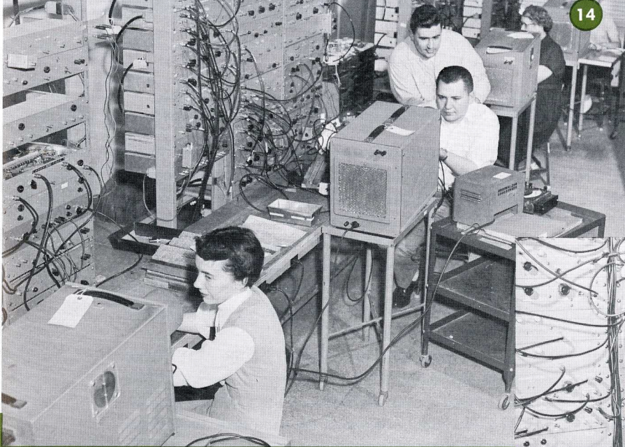
FIG. 14—Manufacturing performance test setup for logical devices conducted on 100% basis. Temperature and humidity controlled.
