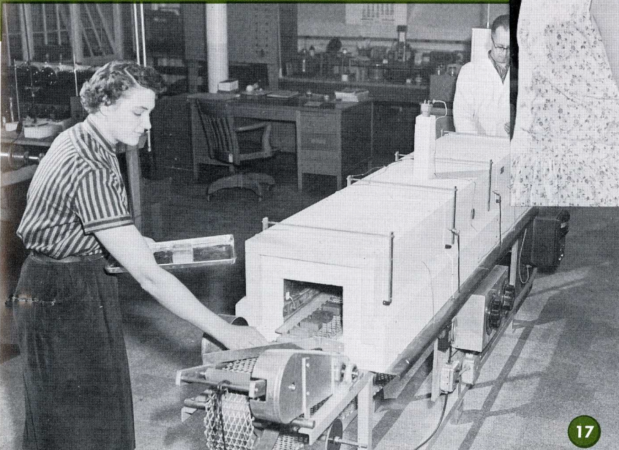
FIG. 17—A continuous curing oven was developed and constructed for controlled runs of encapsulated products.
