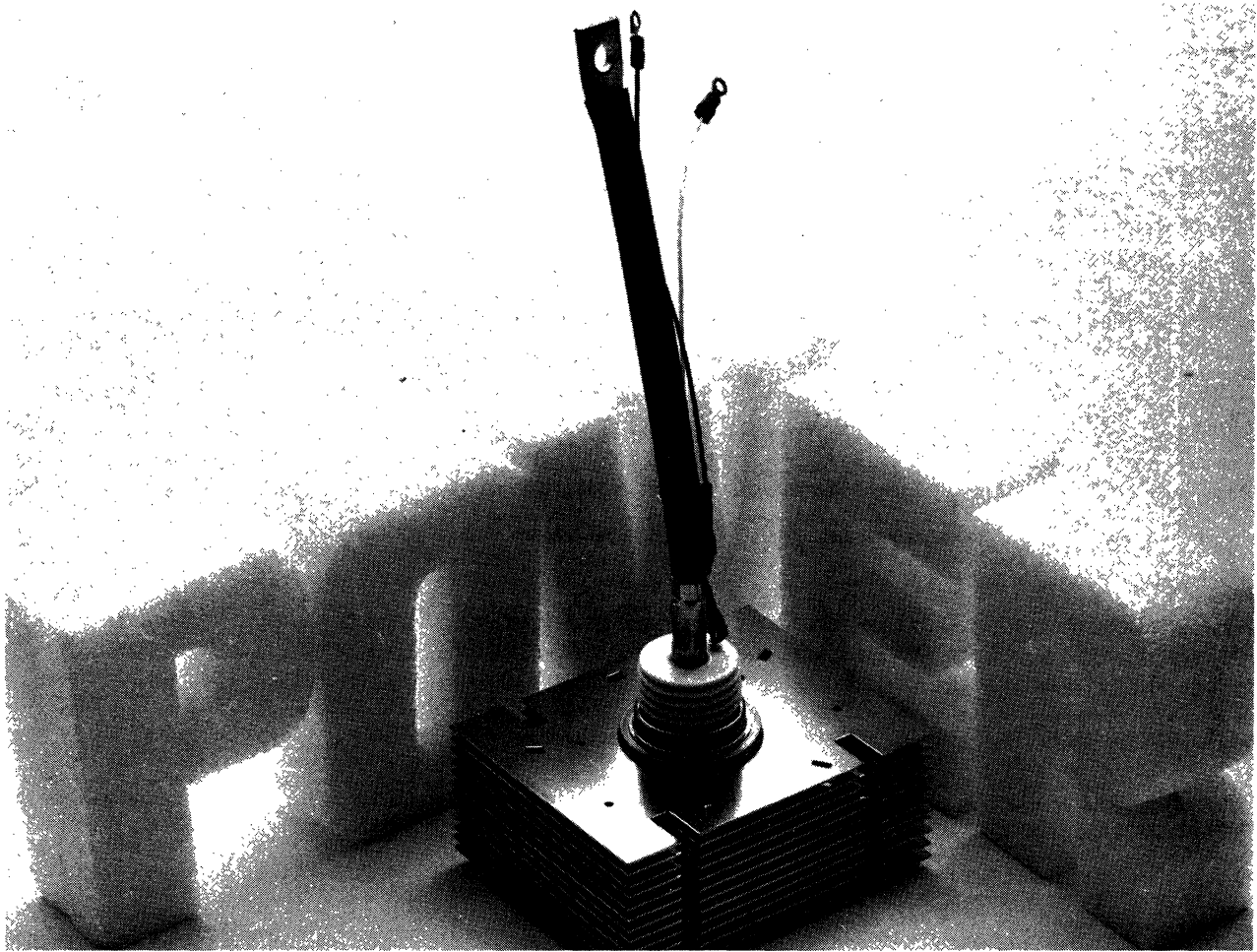
Figure 6.8 An integral heat sink package offers up to a 40% improvement in current rating over the same element size in a stud mount package.
