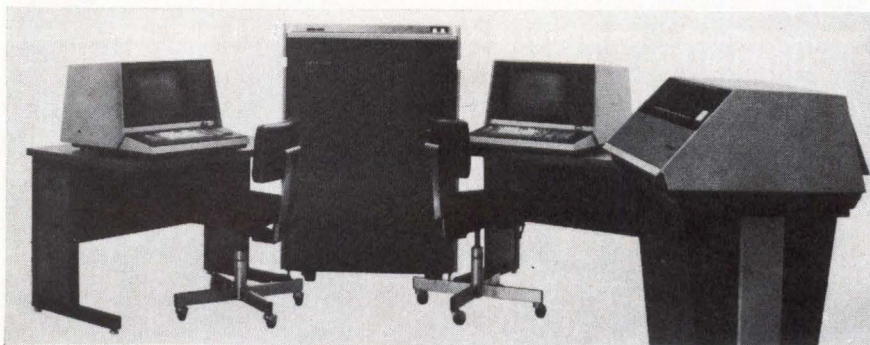
An IBM 3271-compatible online inquiry system, Data 100's model 82 remote display system allows up to 32 stations to perform inquiry, data entry/capture/collection, or other CPU-accessing functions concurrently
