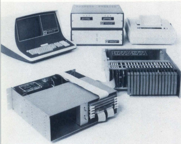
Procom II microcomputer system components (clockwise from bottom left): Procom II, CRT/keyboard terminal, dual mini-cartridge tape deck (top) and Composer, line printer, and RTP universal controller
