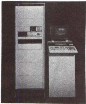
Automatic data acquisition system. Version shown is 3052A system with 9845S desktop computer serving as controller
