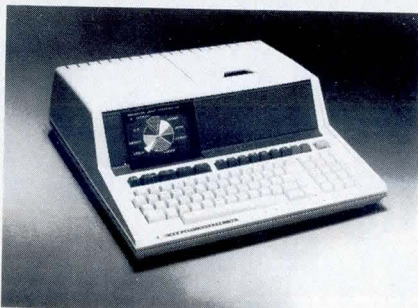
HP-83 personal computer. Hewlett-Packard's typewriter sized unit features integrated keyboard and CRT, plus graphics capabilities
