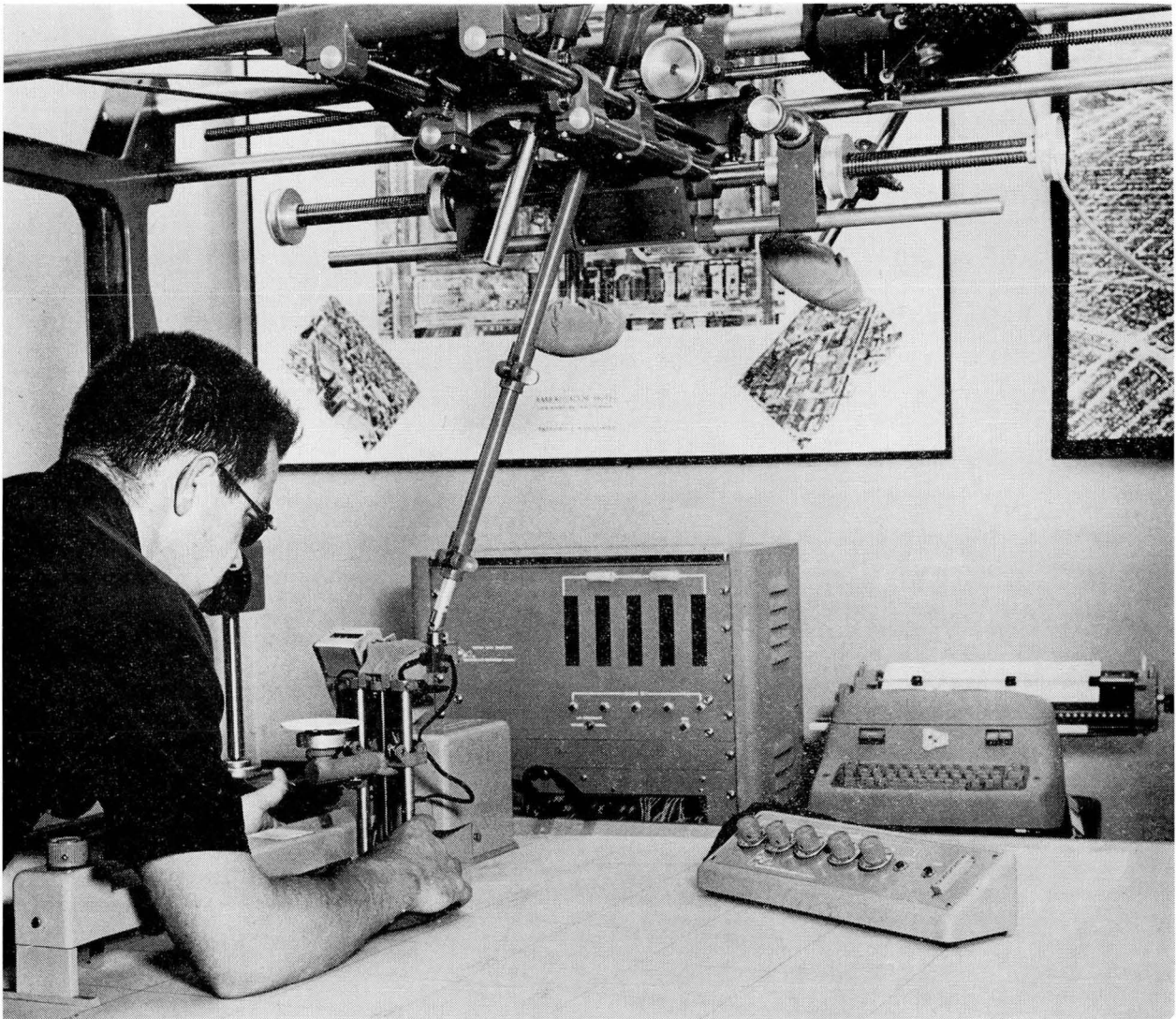
Pictorial information can be converted into digital data for computer input. The machine shown takes stereophotographs and with the aid of an operator converts highway cross-section measurements into digital form punched on punch cards or punch tape. The machine is the Terrain Data Translator made by the Benson Lehner Corp., Los Angeles 64, Calif. (Figure 14)
