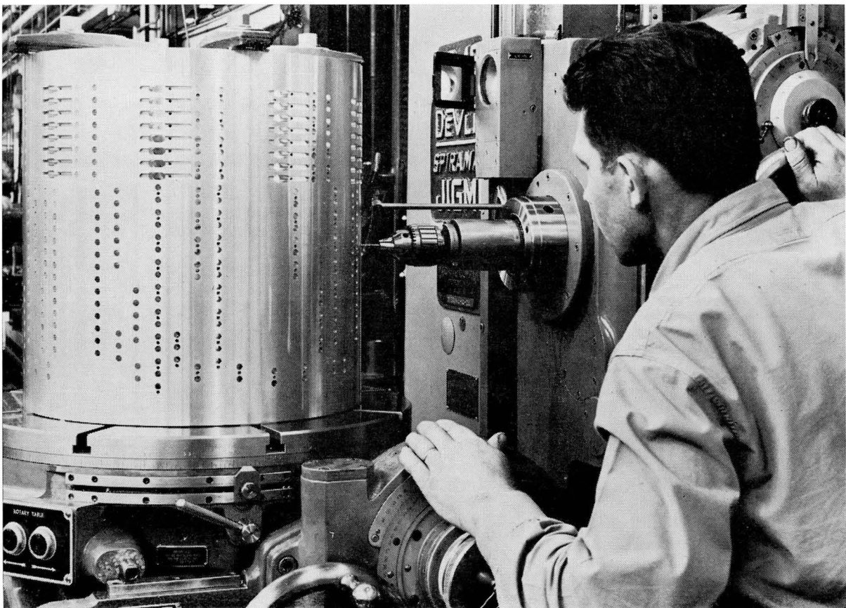
Above the magnetic oxide coating for a magnetic drum is being inspected for concentricity with a micro-probe amplifier. The concentricity tolerance on this particular drum was 70 millionths of an inch. The manufacturer is Bryant Computer Products Division, Springfield, Vermont. (Figure 21). Below holes are being machined into the drum housing in order to fasten the magnetic read/record heads. (Figure 22)
