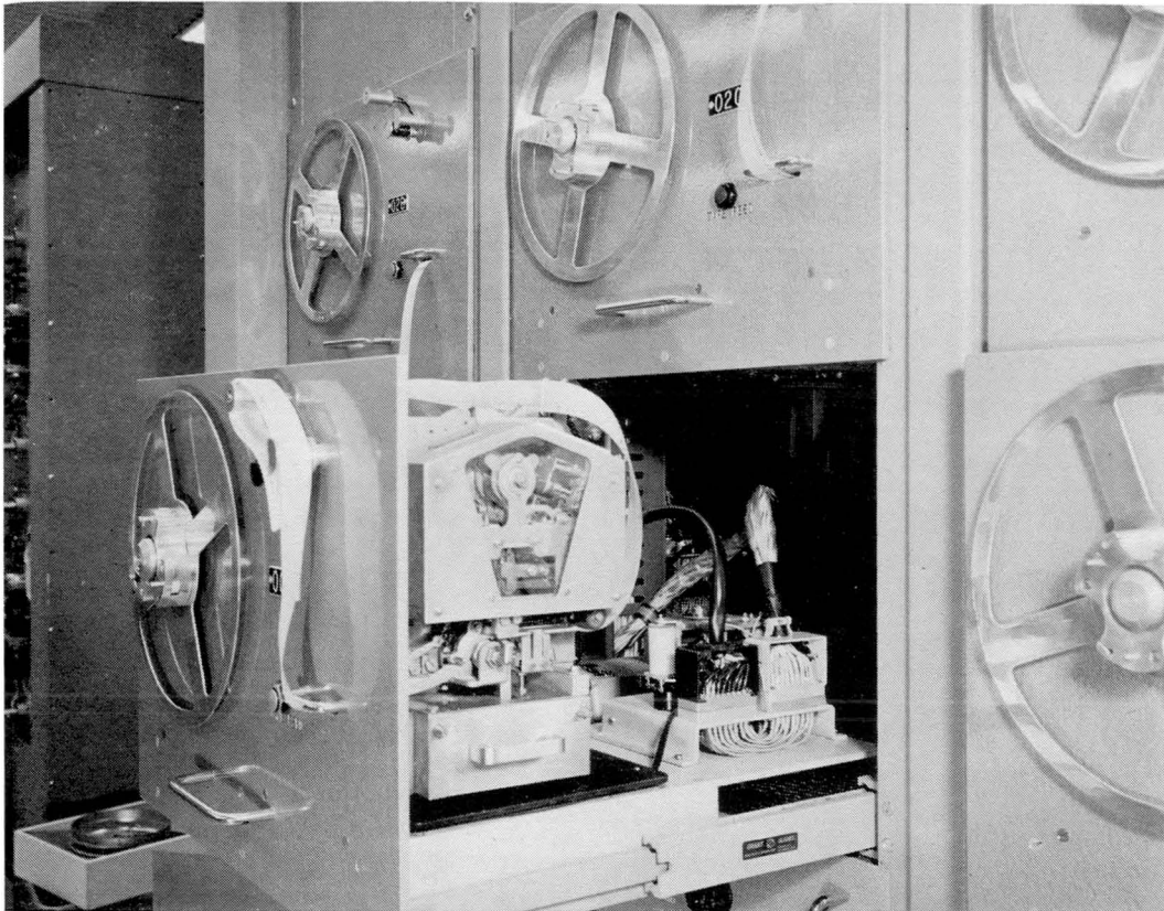
Here is a tape punch which punches 120 characters per second. It is part of FLAC, the Florida Automatic Computer. This machine was designed and is operated by the RCA Service Co., Missile Test Project, Patrick Air Force Base, Florida. (Figure 15)
