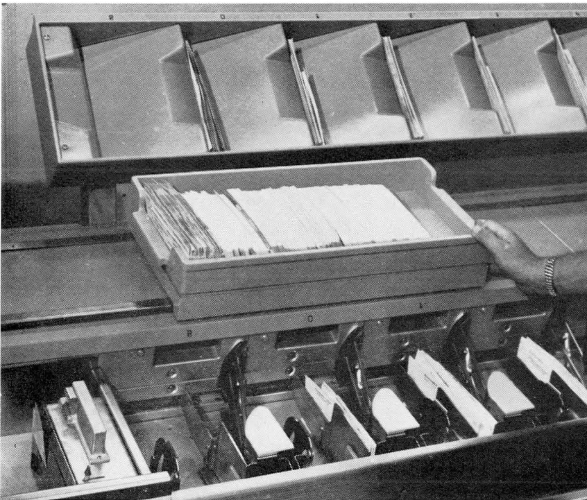
This machine is sorting checks at the rate of 25 a second, by means of magnetic ink characters printed or entered on each check. The characters record account number, amount, and other information. The sorter is an element of the Burroughs B 251 Visible Record Computer made by Burroughs Corp., Detroit, Mich. (Figure 7)
