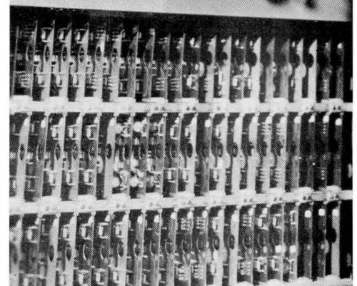
Here is shown a band of Mylar plastic tape containing about 200 instructions for the operation of the Burroughs B 251 Visible Record Computer. Up to 12 tape readers may be installed, so that the computer may refer to more than 2500 programming instructions. Also shown is one of the small transistorized printed circuit boards. (Figure 8)
