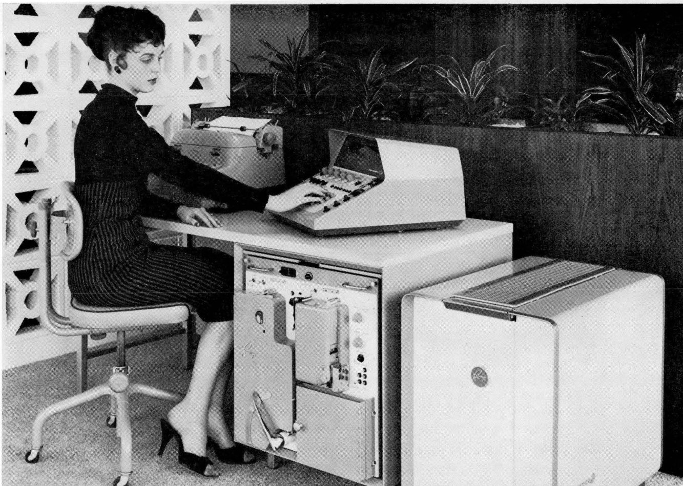
Here is a small general-purpose digital computer, with: electric typewriter input and output; paper tape reader and punch; and at the right, the main computing unit (Figure 9). This is the Recomp II made by Autonetics division of North American Aviation, Downey, Calif. Below is the computer unit opened up. (Figure 10).
