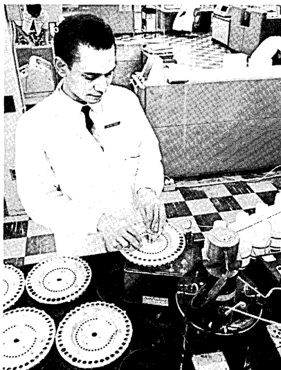
— A technician places blood specimens in an AutoAnalyzer. The testing equipment is monitored by an IBM 1710 computer (background).
