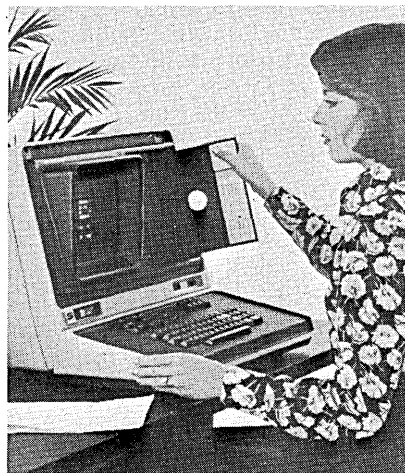
The dual-flexible-disk Model 350 is microprocessor-controlled and has 16k bytes of memory.
