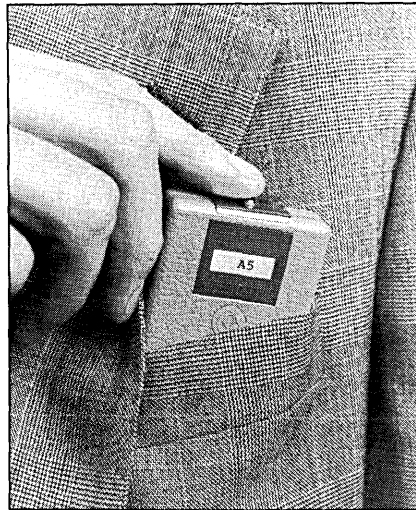
TOKEN: The battery-operated code transmitter sends continuous signals to the control unit, identifying which areas its holder is allowed to enter.
