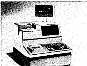
Bubble memory technology provides resident mass memory in the terminal for automatic price look-up for supermarkets and other retail stores.
