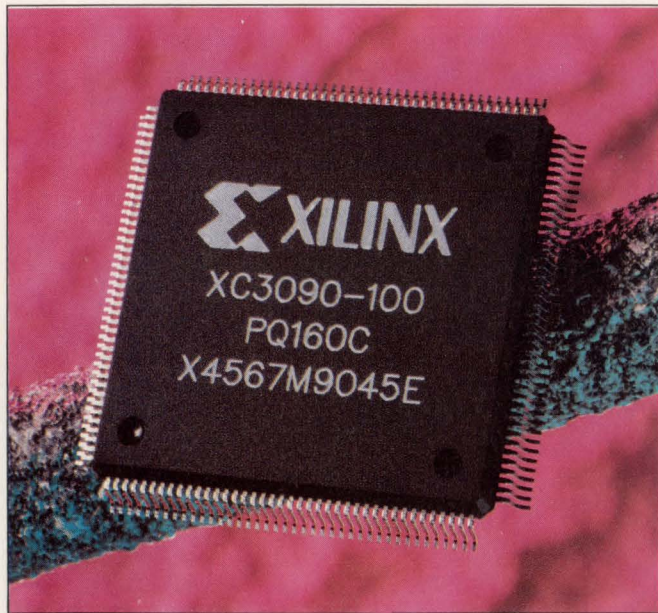
Gate-array-like FPGAs such as the XC3090 from Xilinx typically have excellent I/O resources. This plastic-packaged, surface-device, 160-pin FPGA costs $176.
