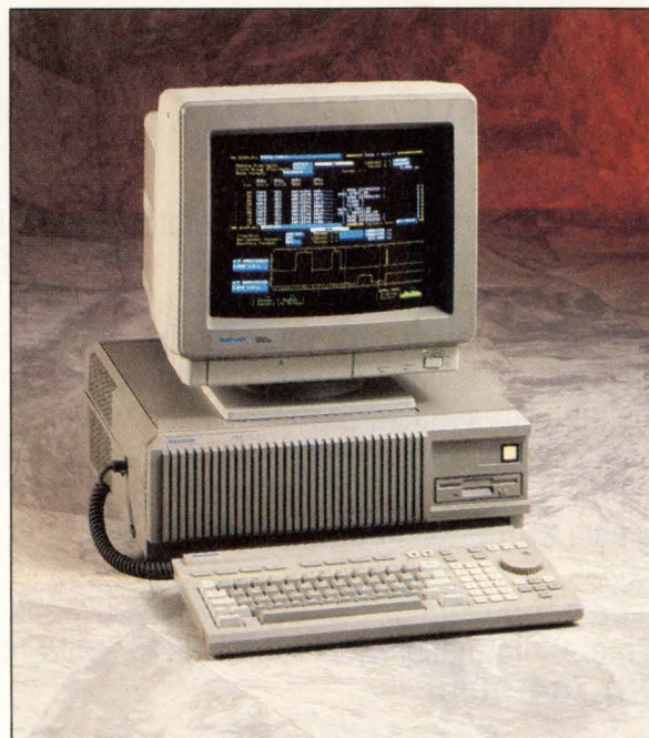
Color displays, available on many combined logic analyzers and DSOs for benchtop use, help communicate information quickly and clearly. Color displays aren't usually available on portables. The Tektronix Prism 3002 is available in several versions, including a portable.
