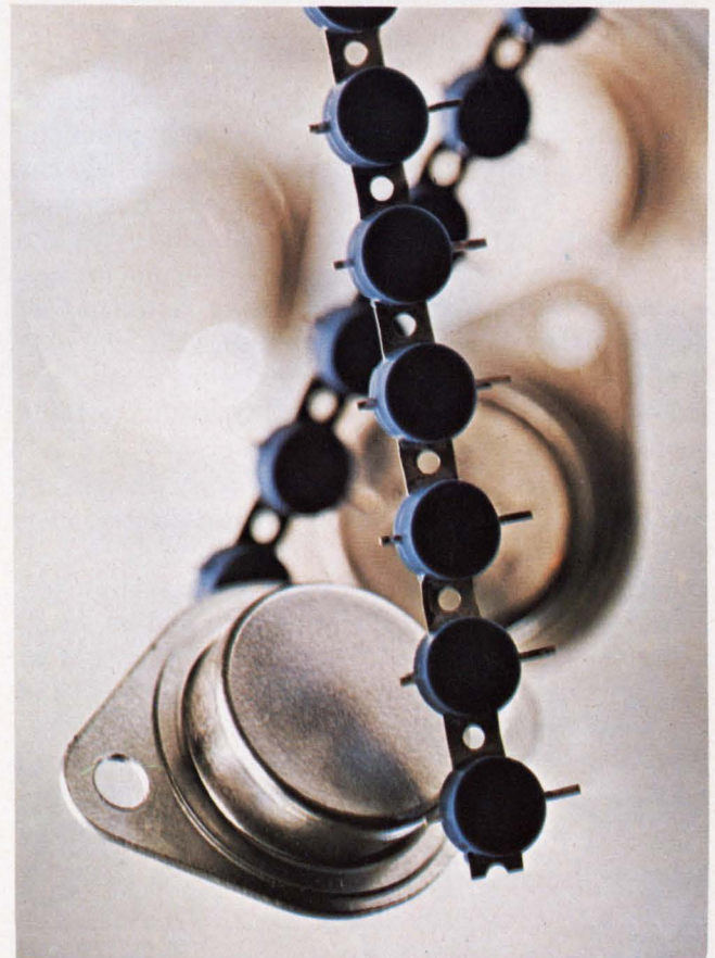
Twenty-five-watt pill transistor molded of silicone dwarfs its metal-can counterpart. Device is Bendix B-5000 power transistor. Material is a Dow silicone.
