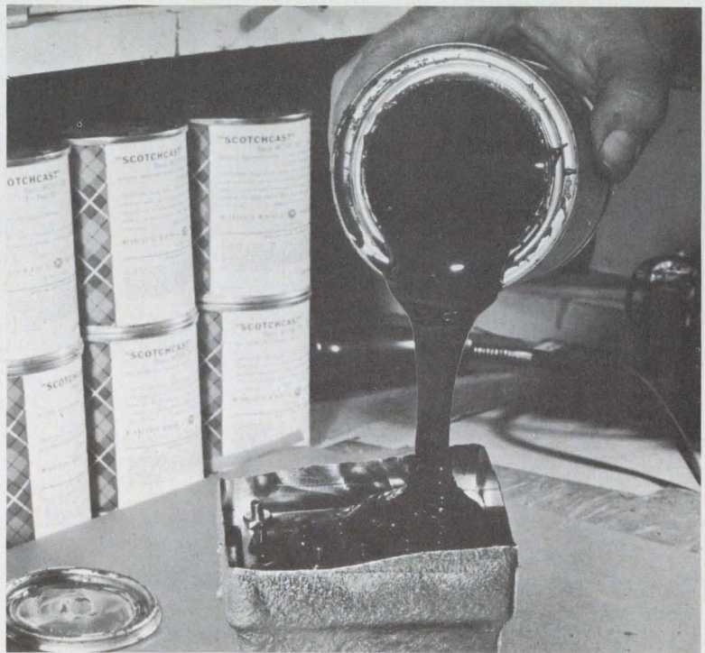
2. Typical casting operation involves slowly pouring the resin-catalyst combination into the mold containing the assembly. A low-cost slush-casting mold is used here to minimize tool costs.
