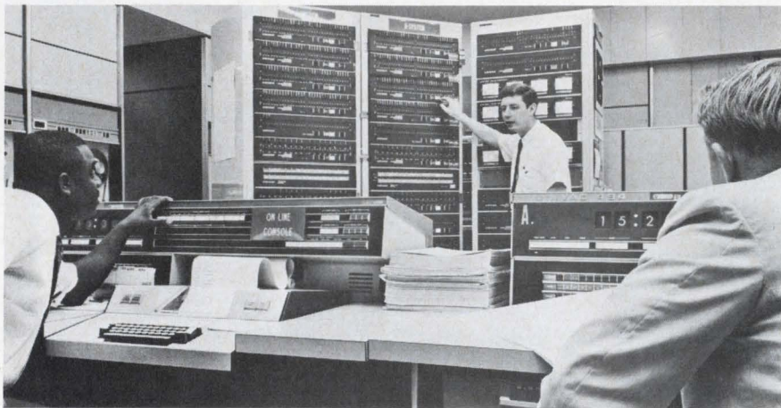
Redundancy is the name of the game. Here, at NASA's Goddard Space Flight Center one Univac 494 is actually in use, one is on hot standby and a third is off-line backing up the other two.
