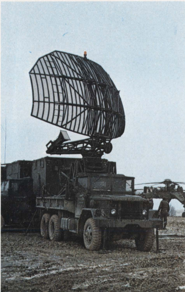
AN/TPS-44 search radar, built for the Air Force 407L air control network, is operating satisfactorily.
