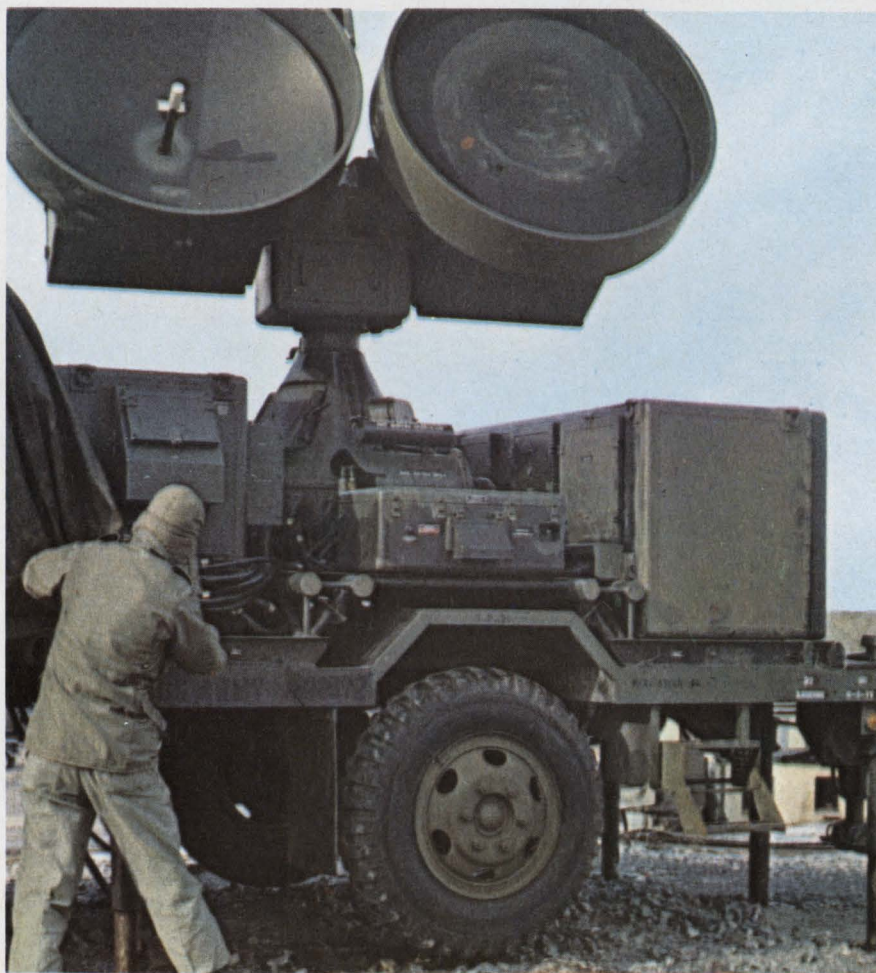
High-powered illuminator radar, (Hipar) illuminates enemy aircraft with electromagnetic radiation on which the ground-to-air Hawk missile can home.
