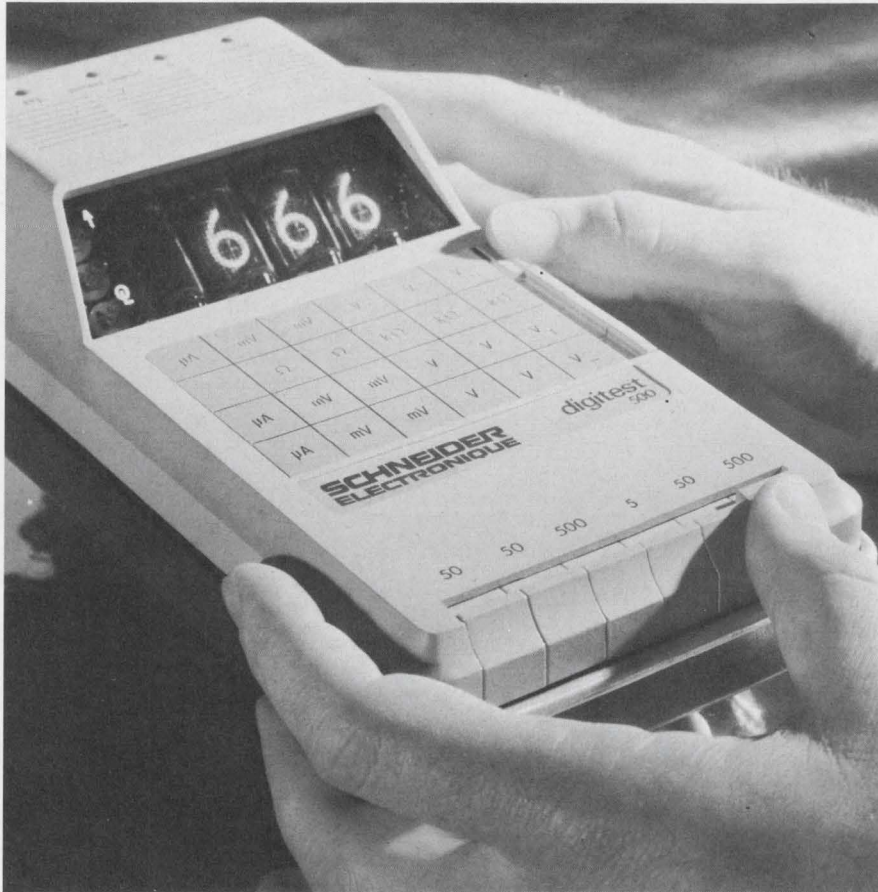
The digital multimeter containing an LSI MTOS chip was a hit at the Paris show. The 2-1/2-pound unit was developed by Schneider Electronique of France.
