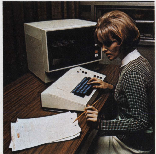
Data communication today: This IBM 2265 display station can be connected to most System/360 computers through ordinary voice telephone lines.
