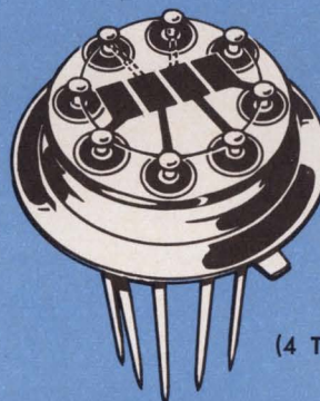
4 POLE 65 MHz TO-5 PACKAGE
