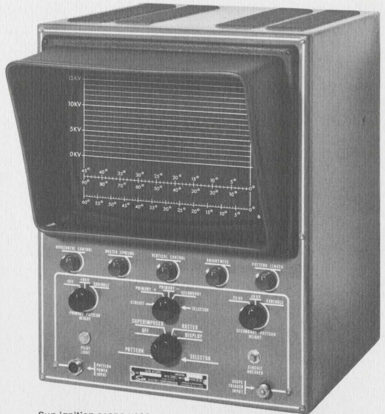
Sun ignition scope uses conventional television picture tube specially modified by Sylvania.
