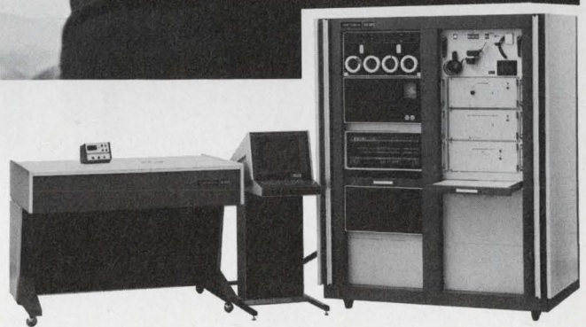
S-3260 Automated Test System
