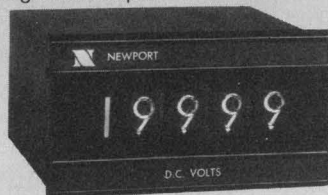
SERIES 2000B DPM: ±19,999 counts • DC voltage and current models 30 rdgs/sec • 2½" H x 4½" W x 5" D. • 0.01% accuracy • BIG-BCD output
