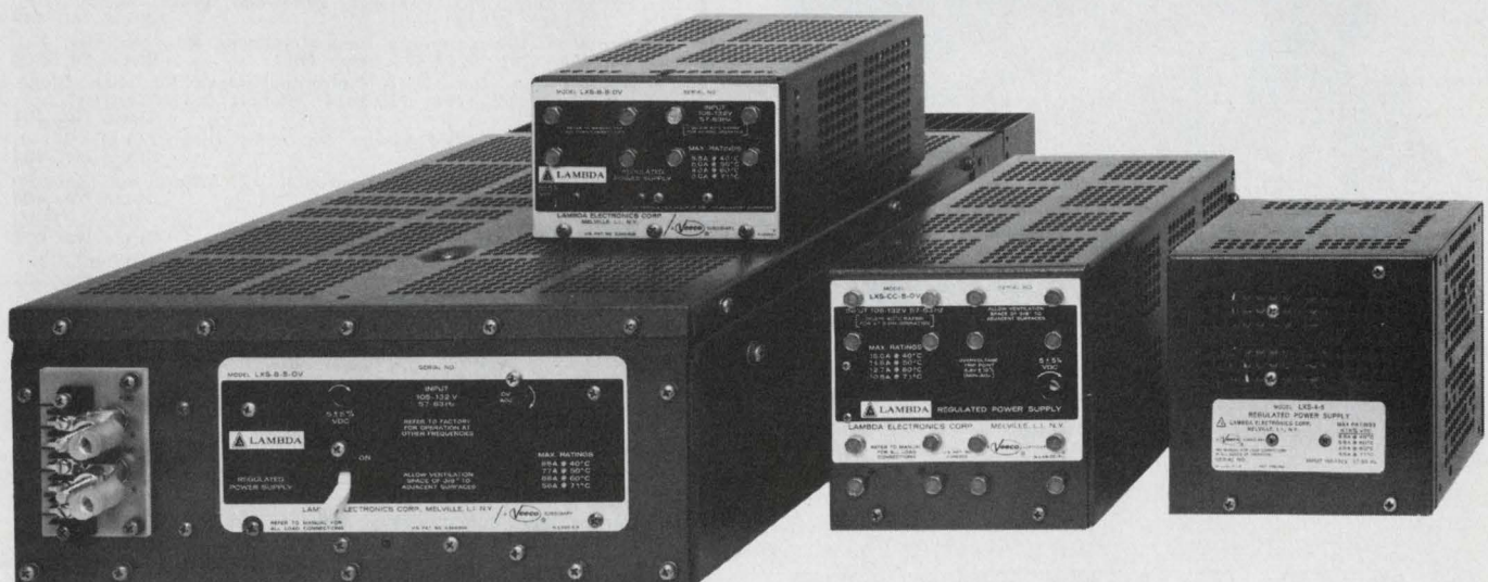
Various models in Lambda's LX Series of modular units output from 35 to 850 W in 10 package sizes.
