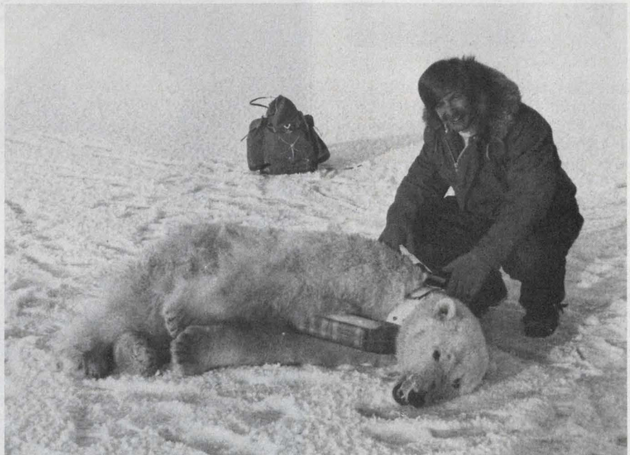
A miniaturized telemetry package that is strapped on to polar bears in Alaska relays a bear's location to researchers via the Nimbus weather satellite. Scientists are studying the effect of the Alaskan pipeline on hibernation patterns.
