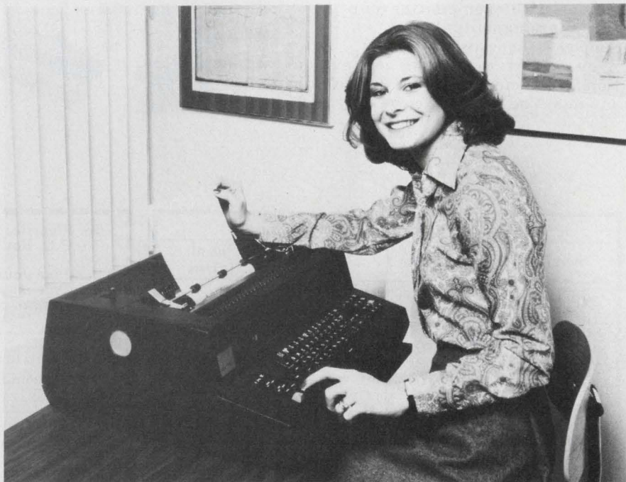
The first electronic typewriter, from the Qyx Division of Exxon Enterprises, distributes computer-aided typing throughout an office while itself taking advantage of multiple processors—three \mu Ps.
