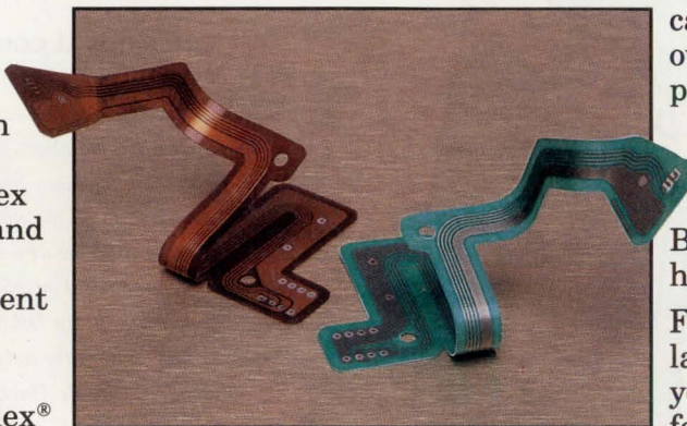
BEND/flex laminates save costs compared to polyimide film circuitry.
