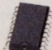
HI-549. Differential 4-channel with dielectric isolation, overvoltage protection, and R_{ds\ ON} matching.
