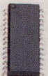
HI-547. Differential 8-channel with dielectric isolation, overvoltage protection, and R_{ds\ ON} matching.
