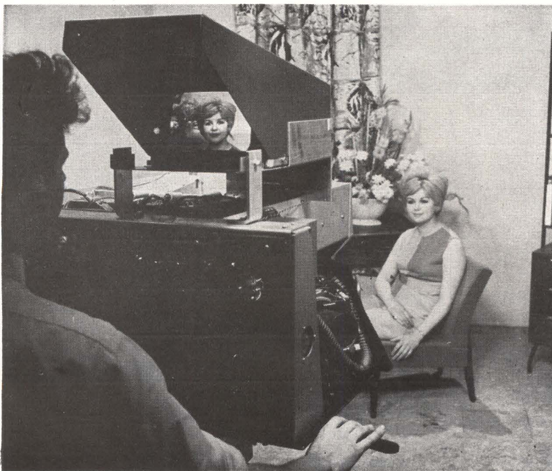
COLORFUL young lady in multicolor dress is used by Marconi during London demonstration of new separate-luminance color-tv camera. Marconi says camera is suitable for NTSC, SECAM and PAL systems. It uses three \frac{1}{2} -inch image orthicons, for luminance, red and blue signals. Green is derived from these three signals
