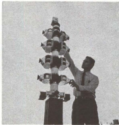
AIR-COOLED power klystron is assembled by Amperex's John Nielsen. Transmitter will be installed in zig-zag antenna, at new uhf-tv site
