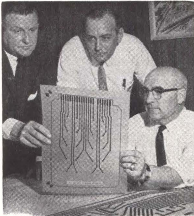
MYLAR MASTER replaces three drawings formerly required to photo etch boards
