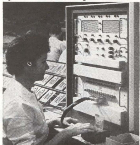
Figure 5 and 6. New welded package Figure 8. TI Model 659A integrated circuit tester
