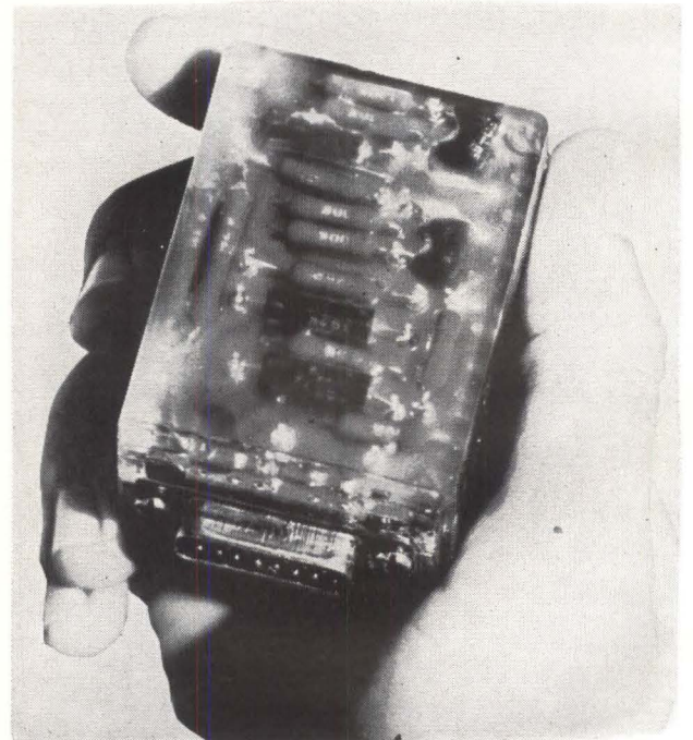
OSCILLATOR used in telemetry system of the Q-2C jet target drone employed by Navy and Air Force for testing ground-air and air-to-air missiles. Designed to withstand 25 water landings and recoveries, the unit has been encapsulated in a room temperature vulcanizing clear silicone elastomer supplied to the manufacturer, Dorsett Electronics, by General Electric. Besides absorbing vibration energy, the silicones serve as short-term high temperature, insulators. Components can be cut out and replaced
