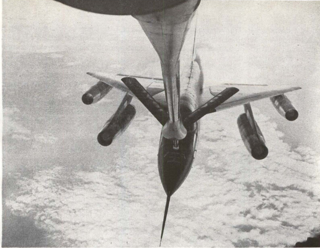
AERIAL refueling of the B-58 Hustler by a KC-135 tanker could not be achieved in an area of clear air turbulence (USAF)
