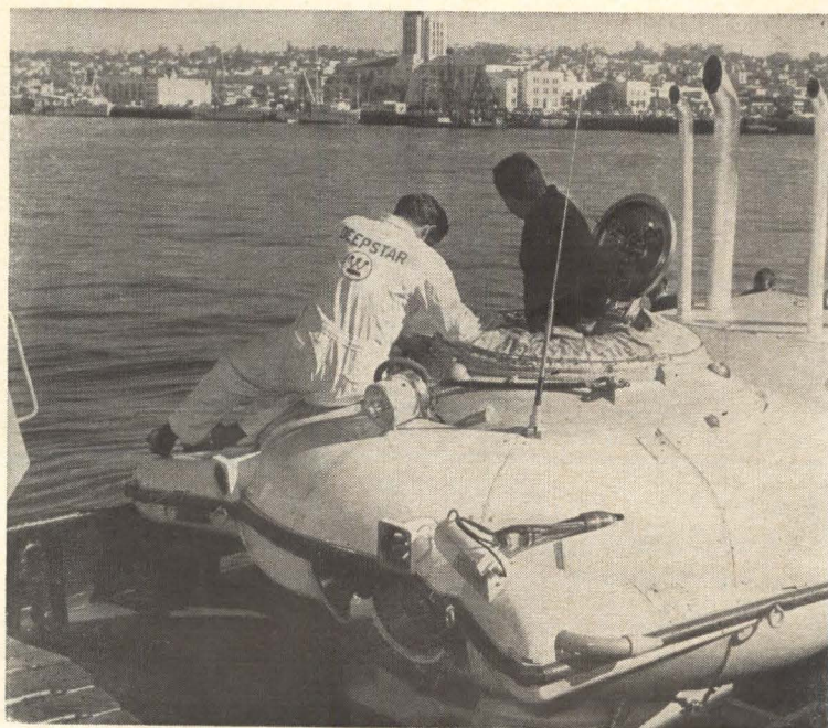
Diving Saucer, being prepared for a test at San Diego, Calif., has a 1,000-foot capability.
