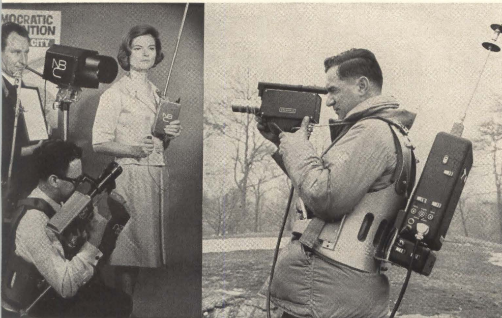
An NBC convention crew shows off its new equipment. Cameraman (kneeling) peers into viewfinder to see girl member of the floor crew holding a microphone and audio transmitter. Man at left, supplying light for tv picture, stands near cone of black-beam audio transmitter. Doghouse with lens, in background, is a black-beam pickup device normally located on a balcony. Picture at right is a self-contained television station weighing less than 30 pounds. It will be used by ABC at the national convention.
