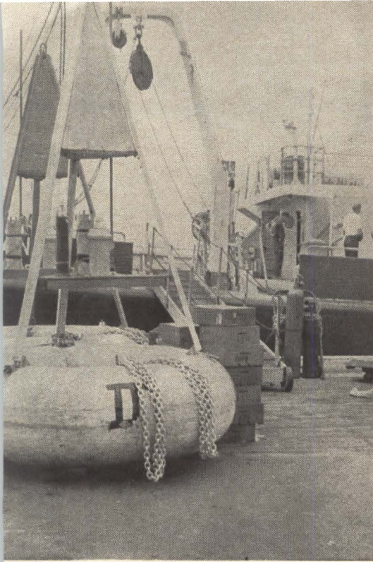
Oceanographic buoys are loaded aboard the Atlantis II. These buoys are fitted with a radar-actuated xenon flash lamp to help in locating them at night. The ship, designed for oceanography, has a steam-powered trawl winch with seven miles of cable. She can accommodate a crew of 30 and a scientific party of 25. She's 210 feet long, 44 feet wide, displaces 2,300 tons and can travel 8,000 miles at 12 knot.
