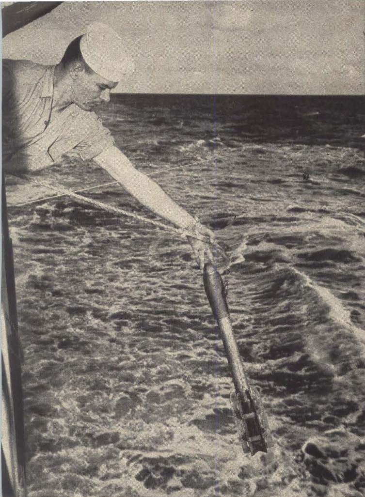
BT WINCH plunges hundreds of feet of wire, with a bathythermograph attached, into the sea.
