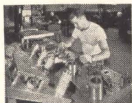
"Modular" setup proceeds rapidly with these reusable components.
