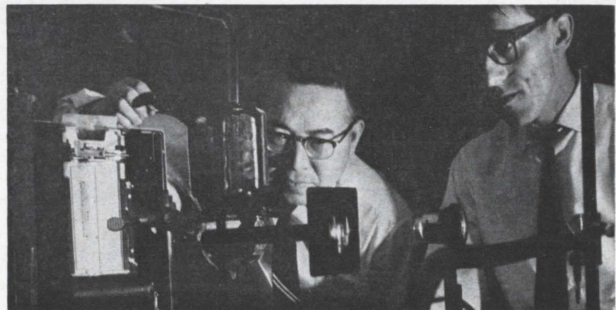
Laser beam created a predicted chemical reaction. Yo-Han Pao (left) and Peter Rentzepis polymerized a monomer molecule.
