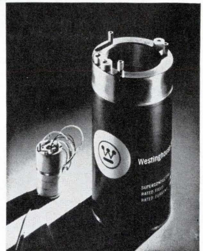
Typical wire-wound superconducting solenoids. Although both magnets have the same rated field, there is a 10:1 ratio of working volume between the large and small solenoids.
