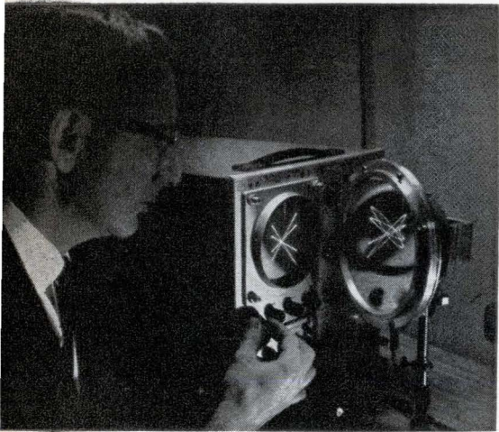
3-D image created by physicist Alan Traub uses an off-the-shelf loudspeaker and a Mylar mirror.
