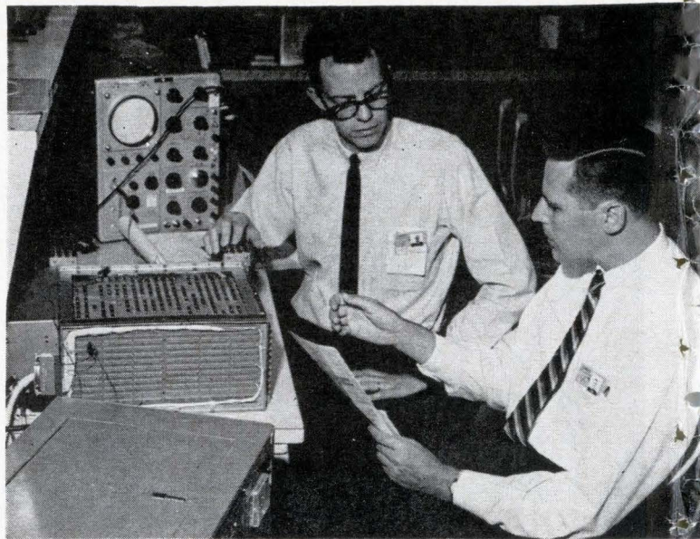
Digital system research model, on the table, contains approximately 5,000 logic gates. Nine two-sided printed circuit assemblies are plugged into a connector card, left foreground, facing the reader.
