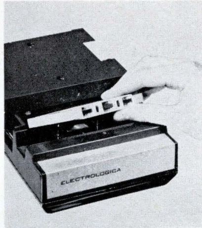
Tape cartridge removed from Intometer recorder later is run through high-speed reader that feeds data from tape directly into a computer.
