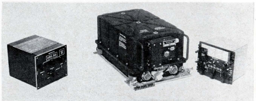
One multichannel ultrahigh-frequency a-m transceiver the ARC 116, left, replaces LOH's two-part ARC 51 which had a transceiver and a control unit.
