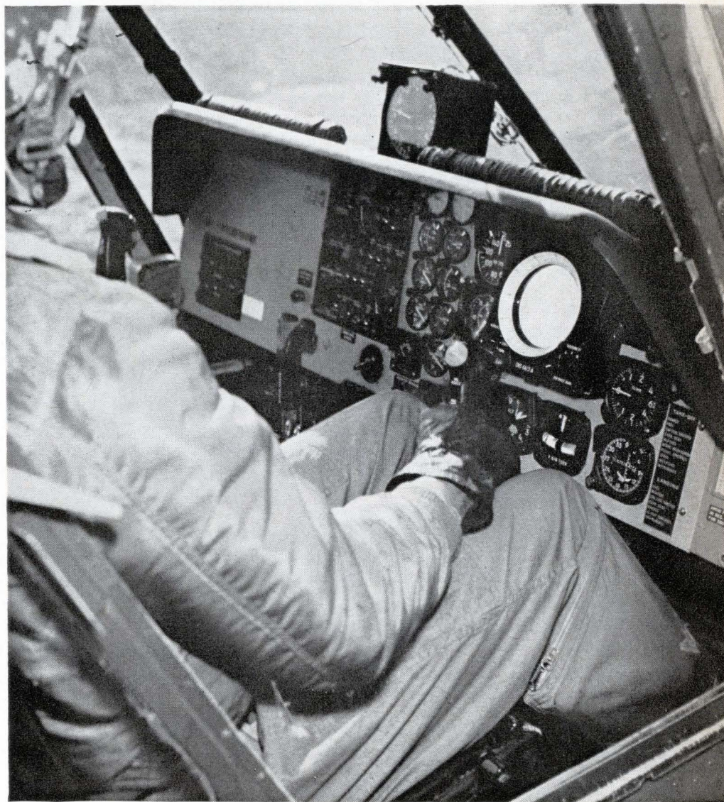
Station-keeping system , developed by the Sierra division of the Philco Corp. The scope in the control panel is the system's plan position indicator.
