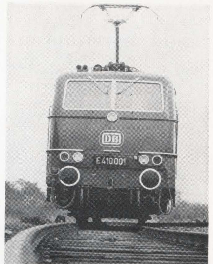
Silicon controlled rectifiers are basis of control circuits in German locomotive that can run on all four European rail power supplies.
