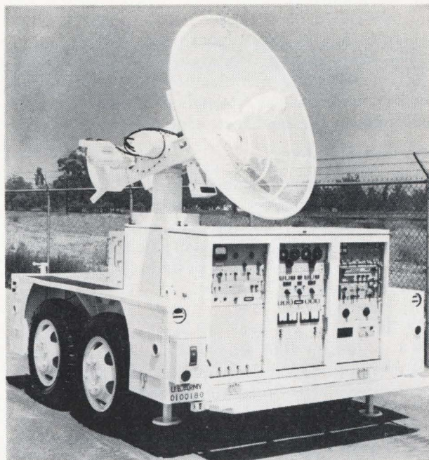
Demand continues high for telemetry equipment such as the Mobile L and S land tracking system built for White Sands Missile Range by Canoga Electronics Corp.
