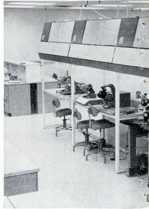
Work stations at American Microsystems are rated class 100.
