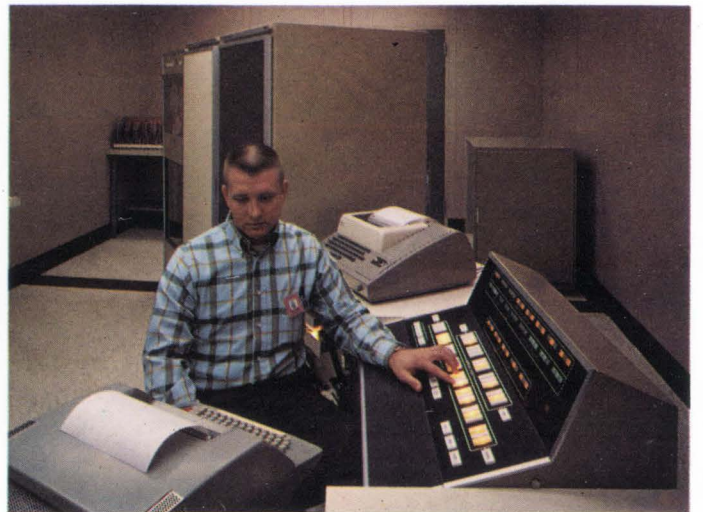
Magnetic tape bearing the routing program from the computer center is used to control a TI 860 computer in generating an interconnection pattern. Here the program data is being checked out on a high-speed printout.
