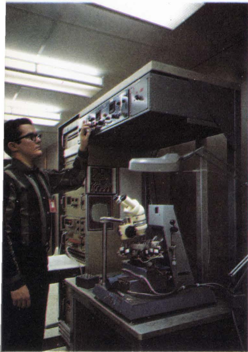
This technician is taking the first step in Texas Instruments' discretionary wiring process, initiating a test sequence on an LSI slice. After optical alignment of probes on a unit cell, the slice is automatically indexed until all cells are tested. Data from test equipment is stored on magnetic tape.
