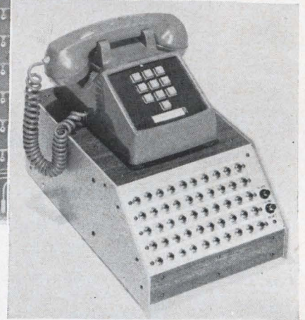
Speedy dial. Automatic telephone dialer can ring a number in seconds. To program the unit, produced by Atlantic Research, the user inserts tiny cubes into a printed-circuit board.
