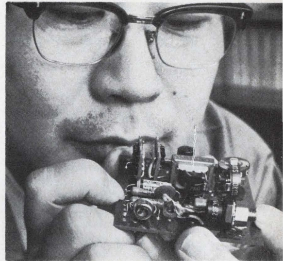
Bright idea. Transmitter for Nippon Electric's laser radar has fewer parts than a six-transistor radio.
