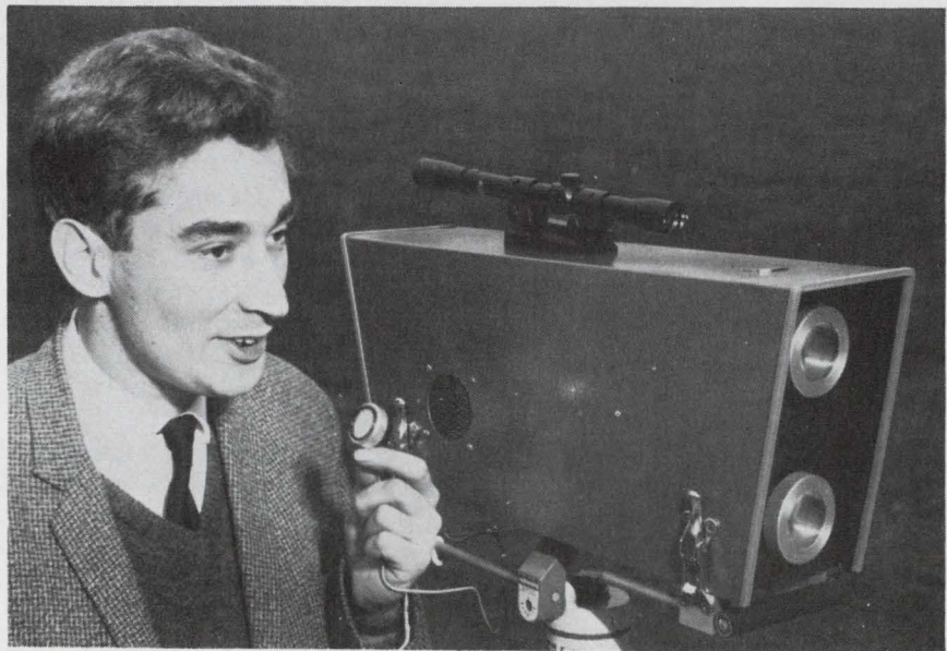
Rig with a yig. Mullard's Roger Cooper talks over infrared telephone link built around the magneto-optic modulator he developed.
