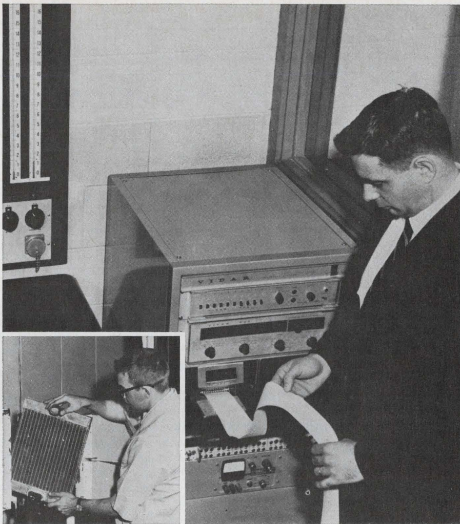
Modine technician prepares test core for wind-tunnel test. VIDAR Digital Data Acquisition System speeds testing of automotive and industrial radiators, oil coolers, and other related products.
