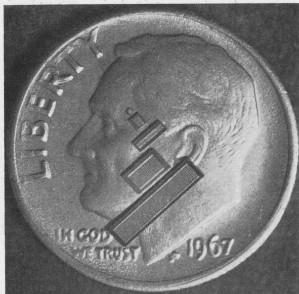
Power pellets. Overlays cover the entire r-f power spectrum. Shown (in order of increasing size) are transistors handling 1, 3, 20, 30, and 100 watts of r-f output power, over the range between 30 Mhz and 2 Ghz.
