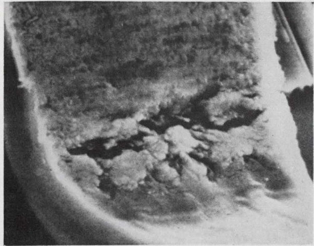
Blowup. Scientists at NASA's Electronics Research Center used a scanning electron microscope to look at aluminum leads ultrasonically bonded to an IC pad. They discovered these transverse microcracks, shown magnified 2,300 times.
