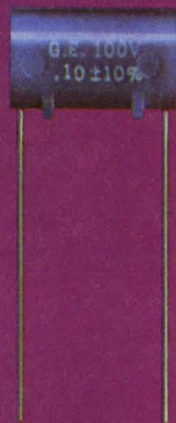
Polycarbonate Tubular Capacitors (left) 64 standard ratings. 100 and 200 volts d-c, 0.001 to 1.0 \mu f, -55 to 85C
