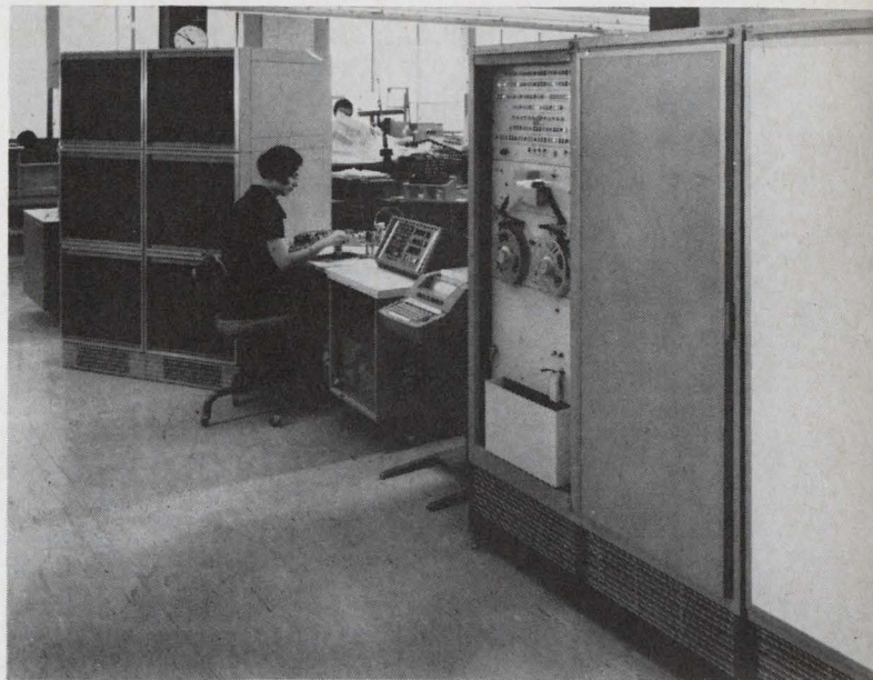
Adaptive system. TI's adaptive tester consists of model 553 dynamic test system and 861 digital controller. The controller keeps track of test results and makes decisions; for example, it stops the test cycle as soon as a device fails any check.
