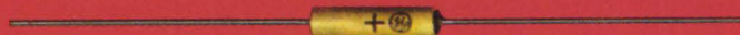
Tantalum Sub-miniature Wet-slug Capacitors 59 standard ratings. 6 to 60 volts, 0.01 to 450 \mu\text{f} , -40 to 85C ambient temperature
