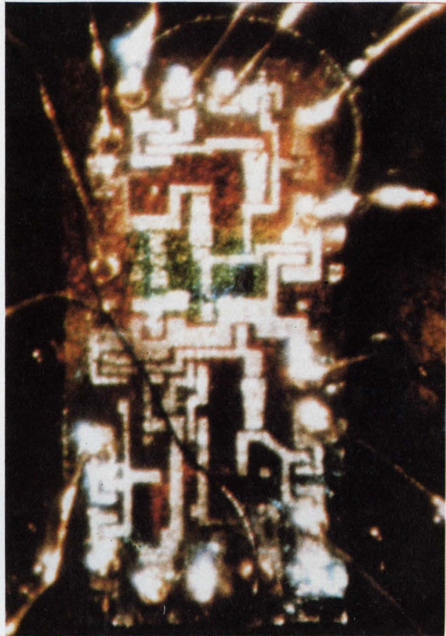
Crystal detector. Hot spots on IC's can be detected with liquid crystals. In the IC above, the hot spot is the blue resistor-diode circuit. The heat dissipation across the IC's surface is shown by the color change from blue to red. The coating, supplied by Liquid Crystal Industries, changes color with minute changes in temperature.
