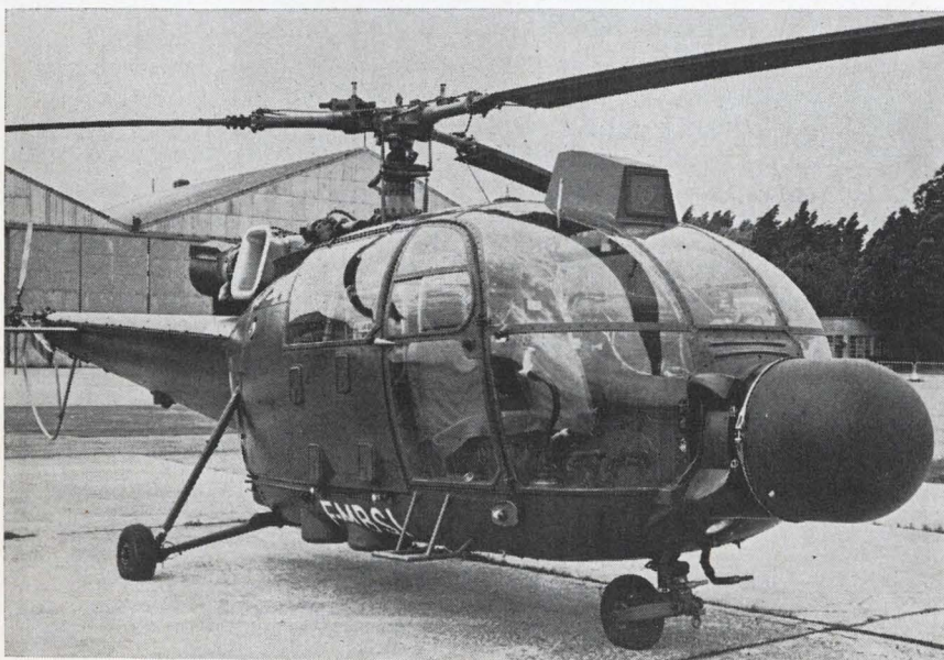
Bulbous. Obstacle-avoidance radar adds a big nose to test helicopter.
