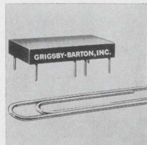
Compact reed relay GB811, in a 14-pin dual-in-line package, is completely compatible with IC logic components and p-c board pin spacing. Input is 5 v d-c for direct transistor logic drive, with the package containing both a reed relay and a diode to suppress back emf. Unit has a contact rating of 3 w. Grigsby-Barton Inc., 107 N. Hickory, Arlington Heights, Ill. 60004. [348]
