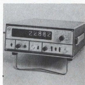
Counter/timer model 1605, for general lab and shop use, measures frequency from d-c to 25 Mhz. Features include input signal conditioning, gate times from 10 msec to 10 sec, 5-digit display with storage and automatic decimal positioning and an internal crystal oscillator with stability of 1 part in 10^6 /month. Eldorado Electronics, 601 Chalomar Rd., Concord, Calif. [368]
