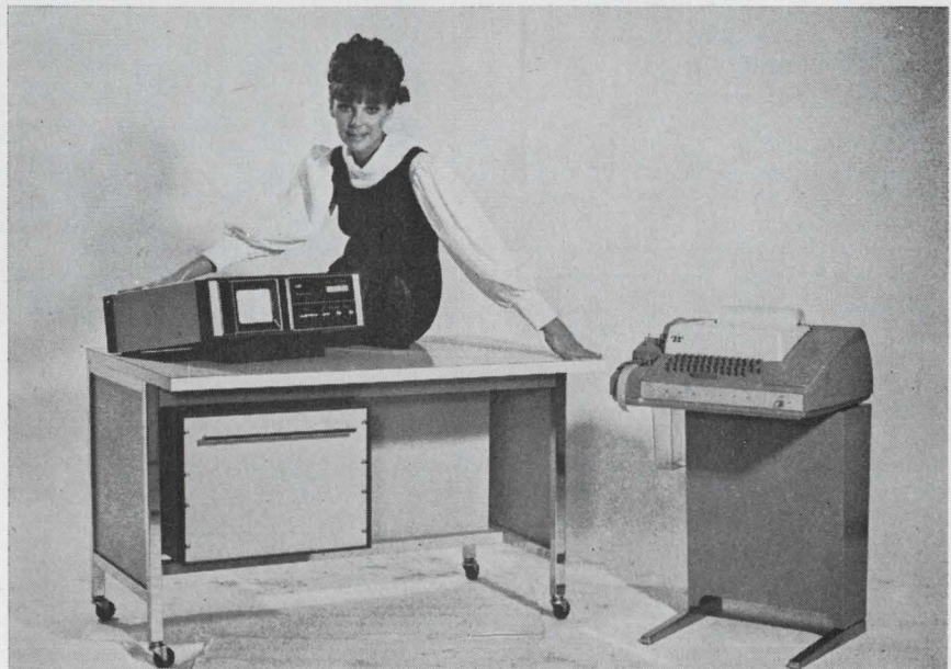
Analyze and display. The CSS-3 processing system includes crt display and teletypewriter printout of the signal components.
