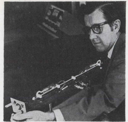
Inspector. He-Ne laser at 10,600 Å is valuable optic-alignment tool.
