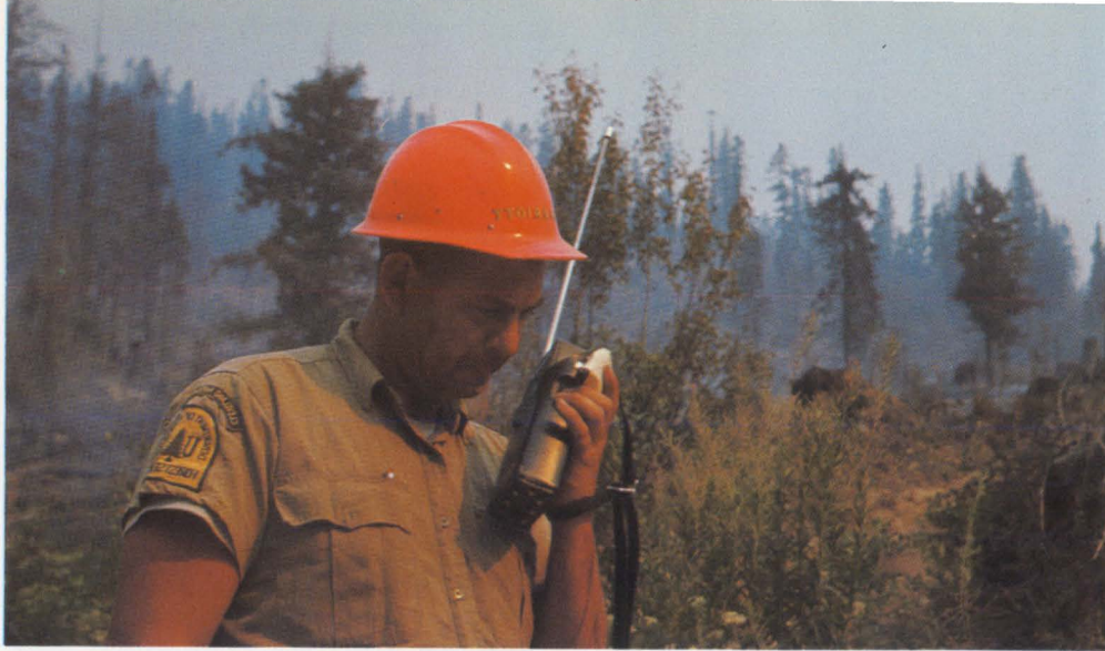
Silvan setting. Small, rugged two-way radios like this Handie-Talkie unit from Motorola are increasingly popular with communications users as diverse as lumber companies and law enforcement agencies.
