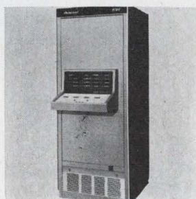
Digital computer DC6024/3 features a full cycle time of 1 \mu sec and a fixed word length of 24 bits. It is for applications requiring real-time control and complex calculations. Basic system includes five 24-bit general purpose registers; an 8,192 word memory; hardware; four levels of priority interrupt; and software. Datacraft Corp., Box 23550, Ft. Lauderdale, Fla. [402]
