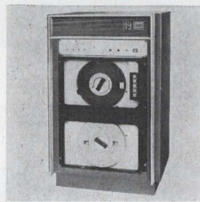
Magnetic tape controller model 119 is IBM-compatible. It contains a 9-track, 800 bpi, continuous read-write magnetic tape transport. It has a reel size of 10.5 in., a continuous tape velocity of 5 ips and a rewind speed of 96 ips. The unit measures 35 15/16 x 24 9/16 x 18 1/2 in. Price will be under $10,000. Daedalus Computer Products Inc., Box 248, N. Syracuse, N.Y. [403]
