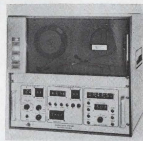
Data acquisition system type DDS1103 accepts bipolar analog voltages up to \pm 10 volts. The data is converted into a 12-bit binary value and recorded in either a binary or BCD format on a synchronous IBM compatible tape. The system includes memory for data collection prior to recording onto tape. Price is $11,250. Digital Data Systems, 18819 Bryant St., Northridge, Calif. [404]
