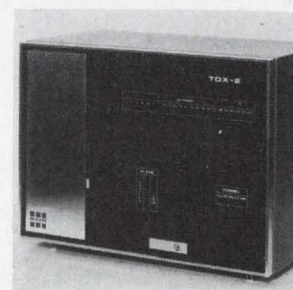
Time division multiplexer TDX-2 can multiplex up to 88 channels with one unit. It will speed intermix up to four rates: 300, 150, 134.49, and/or 110 bps. Status and data quality indicators provide rigorous diagnostic capability. The unit will transmit all combinations of 7 and 8 bit data characters. Rixon Electronics Inc., 2120 Industrial Parkway, Silver Spring, Md. [408]
