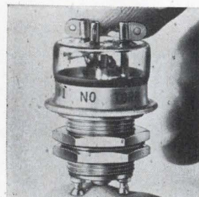
High-voltage, high-vacuum magnetic latching relay TCR/L has a spdt contact configuration and can switch 2,500 w with a 3 msec, 18 v d-c pulse. It can be operated at 5,000 v in air and 15,000 v in oil or gaseous dielectric media. Because of the short pulse used to operate the relay, coil temperature rise is negligible. Torr Laboratories Inc., 2228 Cotner Ave., Los Angeles [347]
