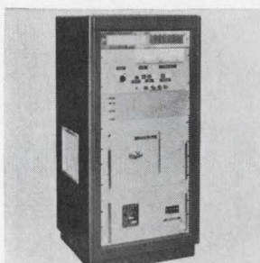
Constant torque a-c variable-speed drive system meets rigid Mil specs. With this system, the exact output speed of the motor shaft can be set and held to 0.05%. Heart of the unit is a digital frequency-control system. A sampling counter senses motor speed every 2.62 sec and compares this speed value to a precision standard. Welco Industries, 9027 Shell Road, Cincinnati [427]
