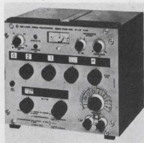
Automatic precision bridge type RLCB can be used for comprehensive resistance, capacitance and inductance component tests over the frequency range 50 hz to 20 khz. It is also suitable for all kinds of impedance measurements. Accuracy for R, L and C measurements is \pm 0.1\% ; dissipation and Q factor measurements, \pm 5\% . Rohde & Schwarz Sales Co. Inc., Box 148, Passaic, N.J. [362]
