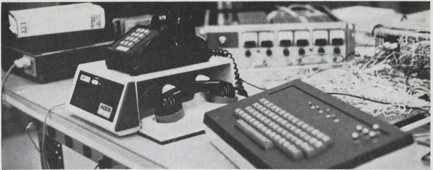
Data by phone. The acoustic coupler is seen under test in the laboratory; a telephone is seated on top of the coupler while a keyboard is used to punch in the desired information.
