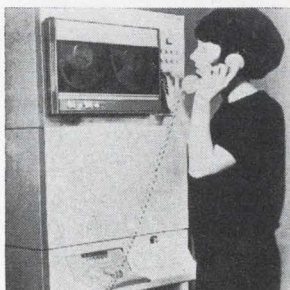
Data-Verter central magnetic tape terminal model 5237 is for gathering information sent over the telephone network from source recorders. It communicates with acoustical or unattended transmitters and records information on IBM compatible 9-channel magnetic tape in ASCII or EBCDIC code. Terminal's rental is under $500 per month. Digitronics Corp., Albertson L.I., N.Y. [405]
