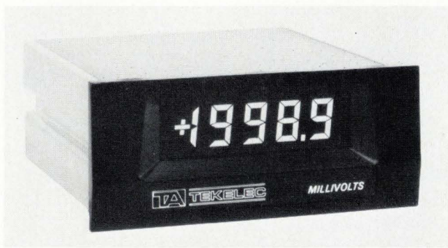
10. Power saver. This Tekelec digital panel meter uses a field-effect liquid-crystal display. Although it requires backlighting, it only needs a 0.5-watt bulb to obtain an excellent contrast ratio.
