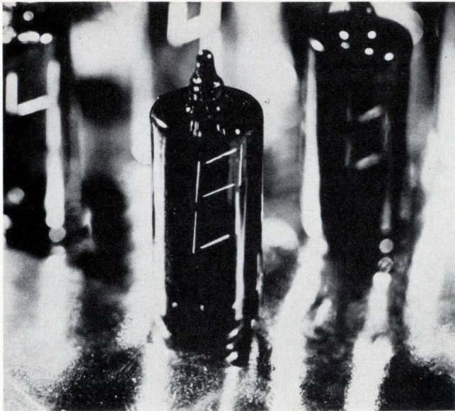
7. The brightest. Where high ambient-light levels are expected, the directly viewed filament display can't be beaten. This RCA Numitron can be made visible under 10,000 foot candles of illumination.
