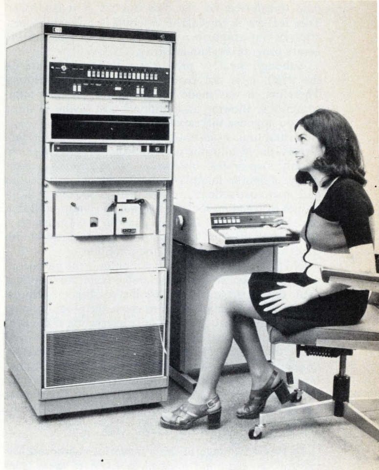
Large. Beefed-up cousin, the H-P 2108A, appears here at the top of the rack in a typical disk-based system. It has a 32k-word memory and nine I/O channels. Both machines are among the first large-scale applications of 4,096-bit MOS memories.
