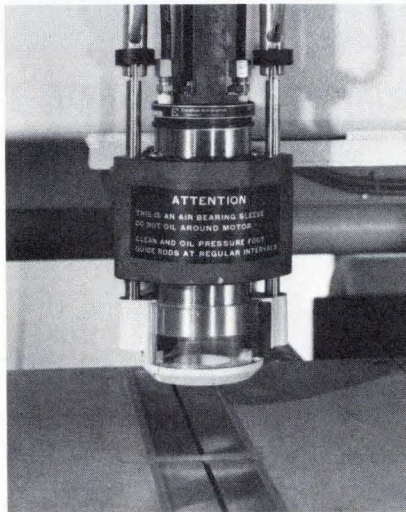
Spindle Assembly with Excellon's Liquid-cooled Quiet Drill Motor.
