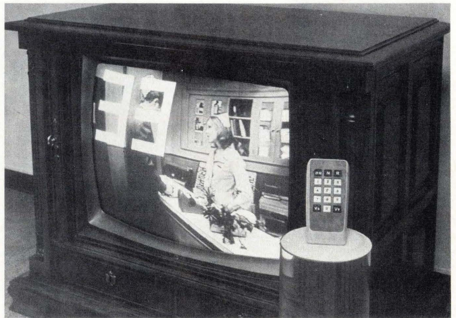
Electronic tuning. Channels are displayed right on the TV screen in Magnavox tuner that replaces electromechanical tuning devices with a portable hand-held remote control set.
