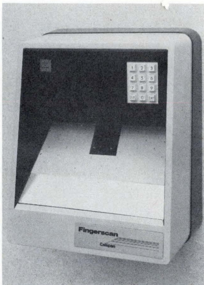
Detective. User keys in number, provides a fingerprint. Fingerscan does the rest.
