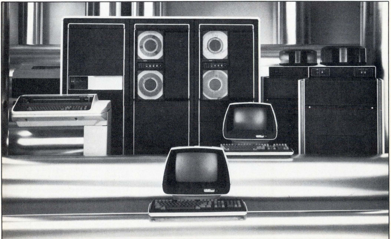
The MV/6000 is rack-mounted and housed in two bays rather than three like the MV/8000.
