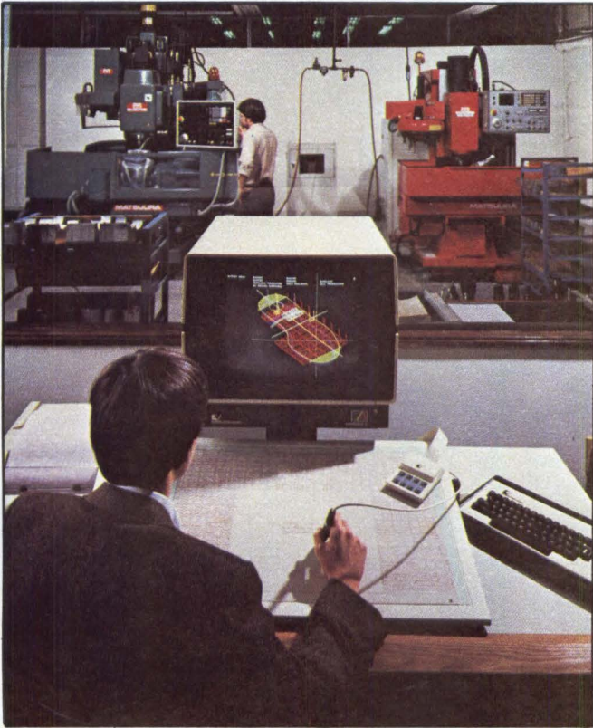
Computervision Corp.'s CAD systems are gaining new interfaces into the computer-aided manufacturing side of the factory. Many vendors that, like Computervision, focus on niche markets in the factory, are beginning to develop software to link their products to the most popular equipment residing in other factory sectors.
