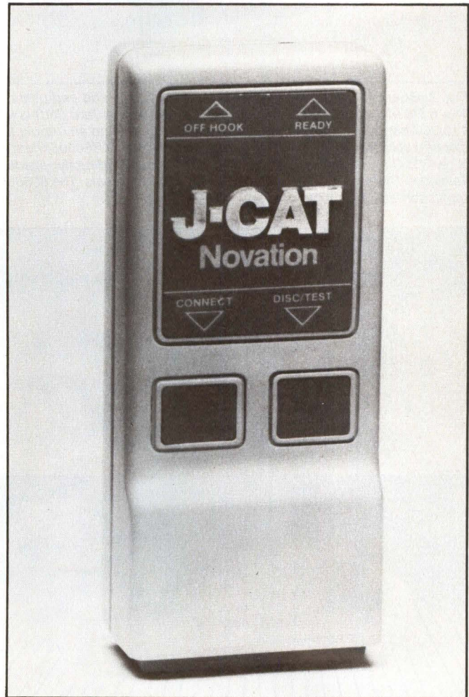
Fig. 1. Novation Inc.'s J-CAT miniature stand-alone modem is approximately one-fifth the size of conventional units. The 300-baud auto-answer/originate modem measures 5 × 1.9 × 1.3 in. and sells for $149. It features LED status indicators, a disconnect/test key, a connect/break key and a beeper that tells a user when a busy signal, carrier or dial tone is detected.
