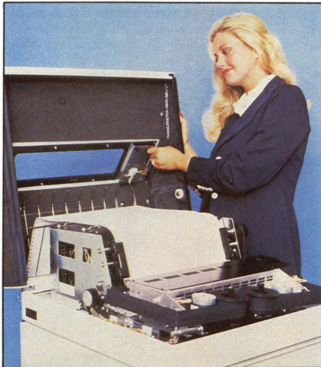
The Trilog TIP-300 line printer prints 300 lpm with two print-head assemblies, features dual-microprocessor architecture and an optional enclosed pedestal and lists for approximately $4900. Single-print-head TIP-150 sells for $3900 and can be upgraded to the TIP-300 for about $1500.
