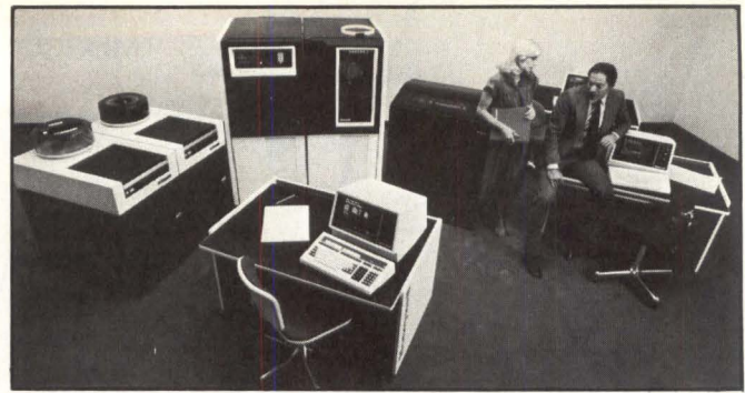
Honeywell Information Systems' DPS/6 32-bit models can be built up from 6-bit models in the field.
