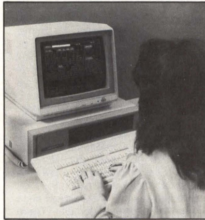
The natural-language package, an option for TI's Professional Computer scheduled for release this year, enables non-programmers to construct database inquiry and other basic applications by selecting appropriate terms from a multi-window screen.
