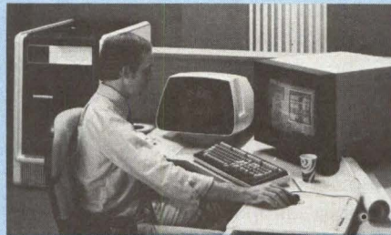
Data General's high-resolution GW/4000 workstation system, which is driven by a 32-bit MV/4000 minicomputer, can display 256 colors simultaneously.
