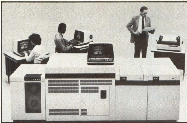
The Wang VS 100 can be field-upgraded from the VS 90 and can be expanded further to 8M bytes of main memory.
