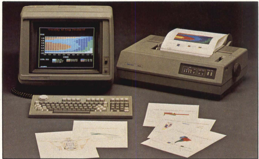
Tektronix's $3995 4105 terminal and the less-than-$2000 4695 color graphics ink-jet "copier" are intended for technical and professional users. The 4695 provides 120-dot-per-in. resolution and six-color images. The 4105 has a 480- × 360-pixel resolution, a 64-color palette and displays 16 colors simultaneously.
