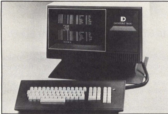
Datapoint 8600 is a desk-top 16-bit minicomputer supporting as much as 256K bytes of memory. It can be used as a stand-alone machine or as a node in an ARC network.
