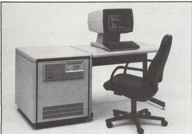
Hewlett-Packard 1000 model A700 is one of the more powerful 16-bit minicomputers with features such as user-microprogramming, 4M bytes of main memory and 12.6M bytes of virtual memory. Its high speed and vector instruction set make it well-suited for engineering applications.
