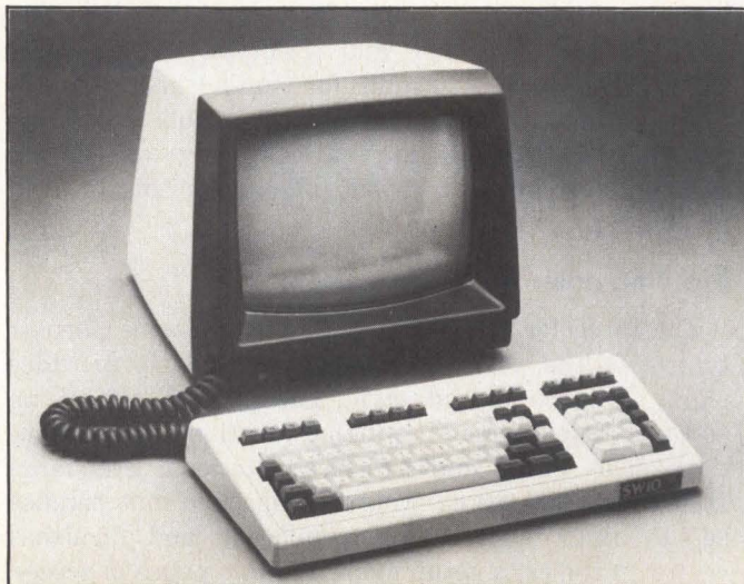
Low-cost but not dumb terminals, the SW10 from General Terminal Corp. (left) and the ADM 22 from Lear Siegler Inc. both furnish 12-inch-diagonal displays, detachable keyboards, setup modes and numeric keypads. The SW10 also provides eight programmable functions, split-screen capability and 11 international keyboards; the ADM 22 provides editing functions and business graphics.
