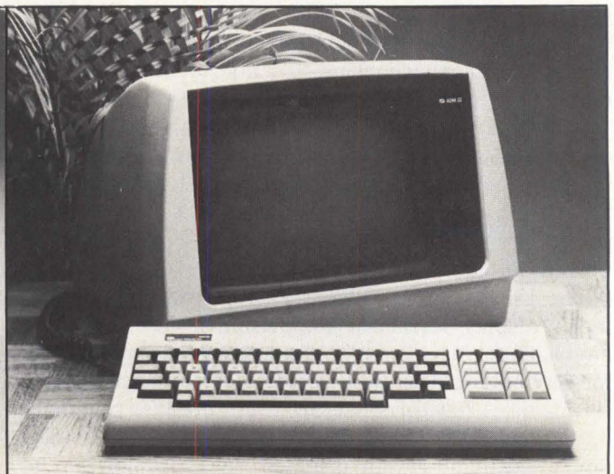
Low-cost but not dumb terminals, the SW10 from General Terminal Corp. (left) and the ADM 22 from Lear Siegler Inc. both furnish 12-inch-diagonal displays, detachable keyboards, setup modes and numeric keypads. The SW10 also provides eight programmable functions, split-screen capability and 11 international keyboards; the ADM 22 provides editing functions and business graphics.
