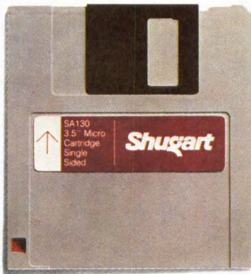
The 3.5" Micro-Cartridge provides maximum media protection.
