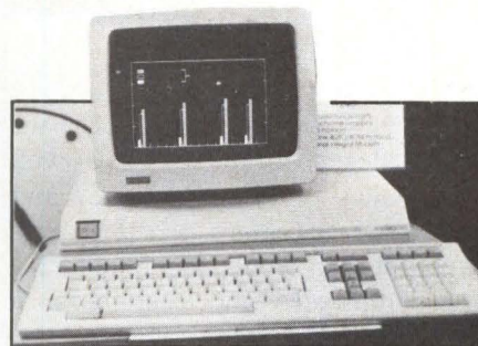
The forthcoming VT200 family includes the VT240, which has the functions of a VT100 terminal, plus a printer port, advanced video, 15 programmable function keys, monochrome graphics and ReGIS and Tektronix 4010/4014 protocols.
