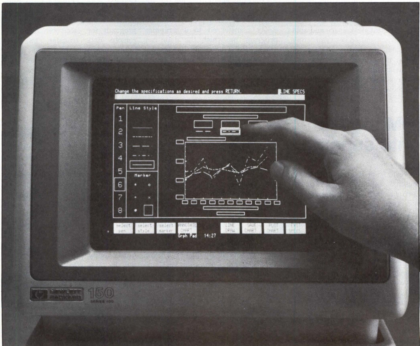
Hewlett-Packard Co.'s HP 150 is its first personal computer aimed exclusively at non-technical markets. Ease-of-use features include eight blocks across the bottom of the touch screen that correspond to the functions of eight soft keys across the top of the keyboard. The system is based on an 8088 processor and runs MS-DOS but is not IBM compatible because of its use of 3½-inch microfloppy disk drives.
