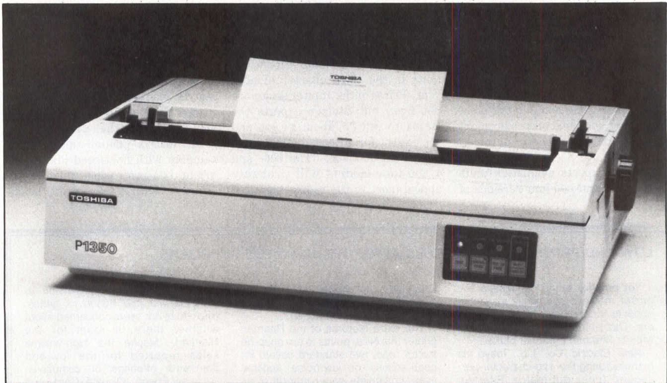
The P1350 from Toshiba America is considered the first successful serial matrix printer in the United States employing a 24-pin print head. Toshiba plans to introduce an 80-column version of the printer this month.
