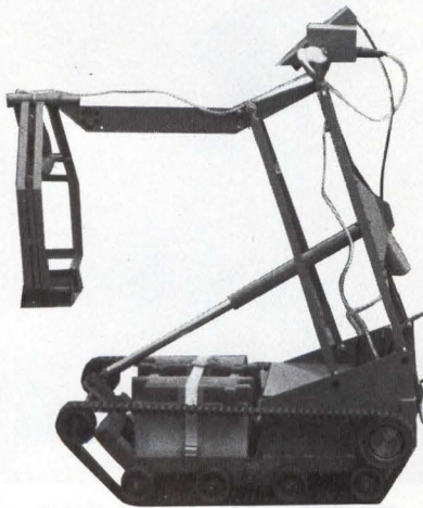
The Navy's remotely operated vehicle for emplacement and reconnaissance (ROVER) can be operated via cable or radio link.
