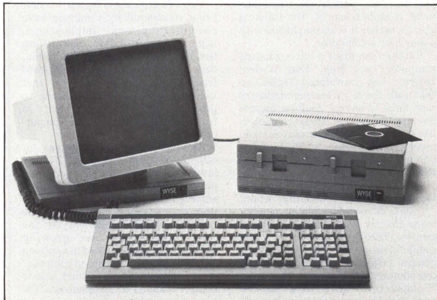
Wyse Technology's WY-1000, based on the Intel 80186 16-bit microprocessor, provides Wyse ASCII terminals, such as the WY-50 (left), with personal computing capabilities. With the $695 WY 50, the package sells for $2,495.
