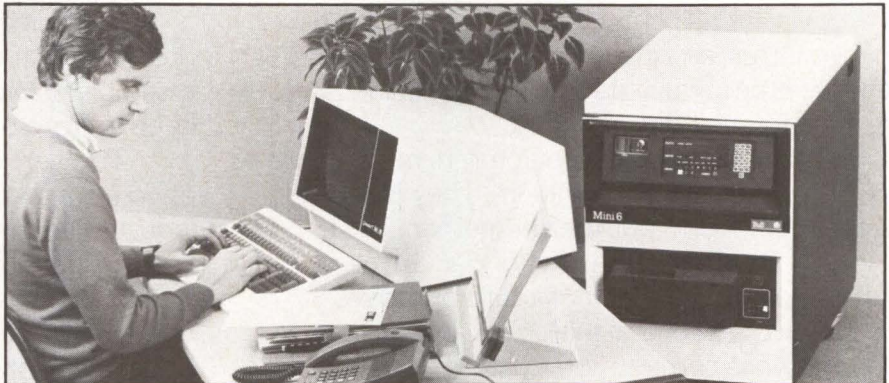
The Mini 6/290 16-bit minicomputer from Bull-Systèmes, Paris, includes 512K bytes of memory, uses the Megabus architecture and, starting in September, will run UNIX Version 7 as an alternative to the GCOS Mod 400 operating system.
