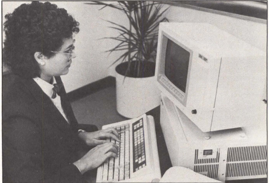
IBM's 9002 multiuser, multitasking desktop microcomputer is based on the Motorola MC68000 microprocessor and has the XENIX operating system available as an option. Price for a configured system with XENIX is $15,960.
