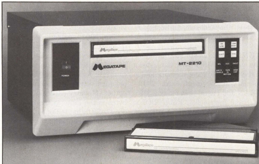
MegaTape's MT-2000 series tape-cartridge drives add capacity by using 1,500 feet of high-coercivity, thin tape. The model MT-2210 (pictured) stores 500M bytes in a book-sized cartridge.
