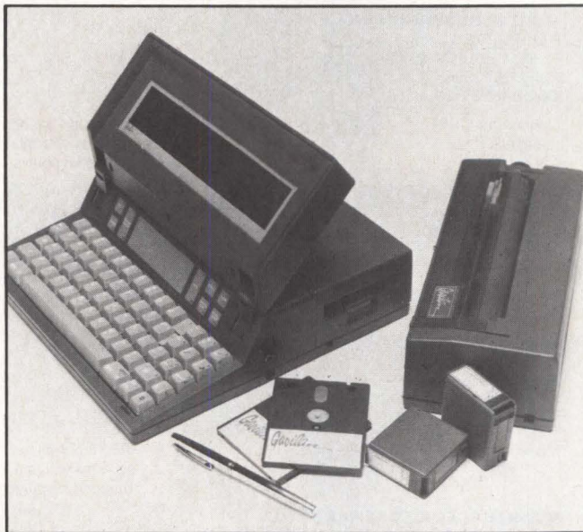
Offering an innovative approach to an integrated system, the Gavilan mobile computer closely couples the operation of software and hardware. It incorporates a touch-panel pointing system for manipulating the cursor.
