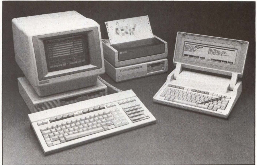
HP's growing family of portable personal computer products can all be linked to its HP150 touch-screen desktop system (left). The Portable (right), the ThinkJet printer (background) and the 9114 disk drive offer a modular system of battery-powered portable devices.
