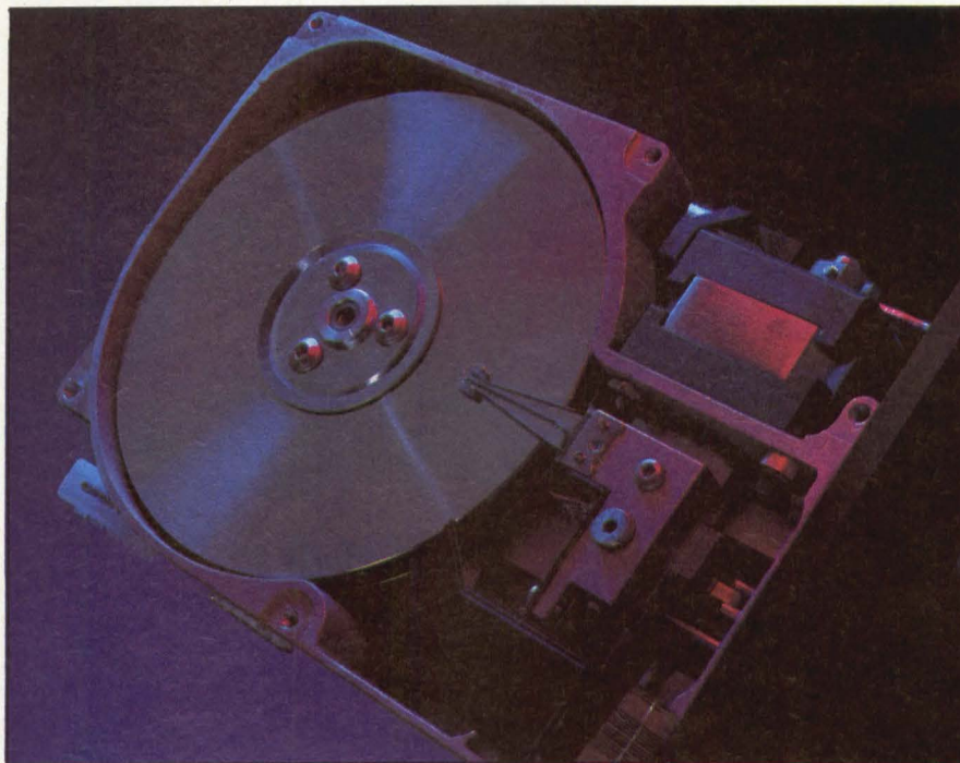
MiniScribe's model 8425 3½-inch drive features 20M bytes of formatted capacity and a single-board ST412-compatible interface.
