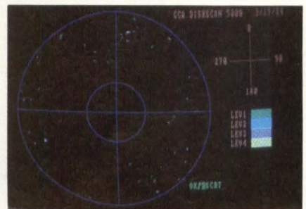
Typical disk defect map.
